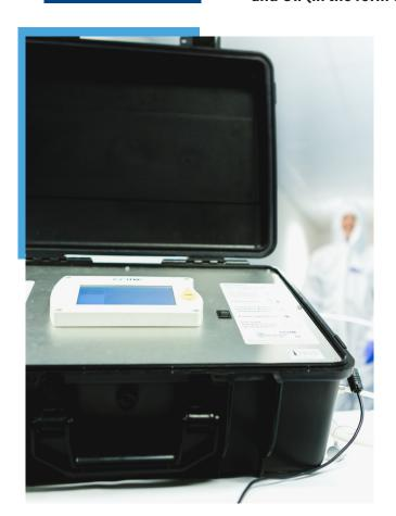
Direct Air & Pipework can measure compressed air to ISO 8573-1 class 1 of the ISO standards.
